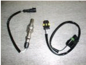
Figure 2 Oxygen Sensor with adapter cable.
